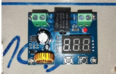
Gambar 2. 14 Low Voltage Disconnect (LVD) (Sumber: dok.pribadi, 2024)
