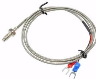
**Gambar 2.5** Thermocouple
