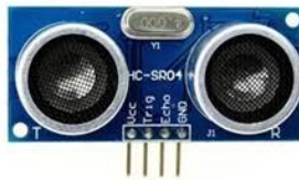
Gambar 2. 4 Sensor Ultrasonik HC - SR04
