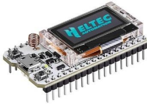
Gambar 2. 10 Heltec LoRa SX1278
