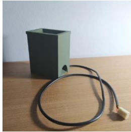
Gambar 2. 20 Sensor Rain Gauge
