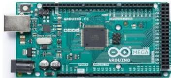
Gambar 2.5 Arduino Mega 2560<sup>[5]</sup>
