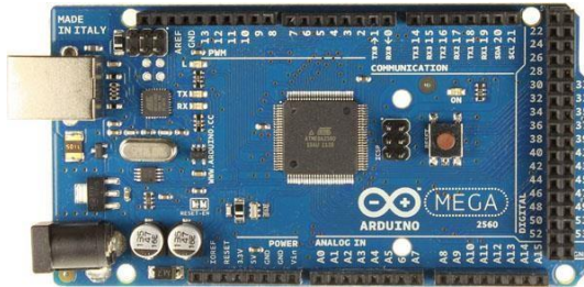
Gambar 2.3 Arduino Mega R3[11]
