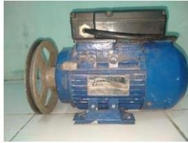
Gambar 2.9 Motor Asinkron[12]
