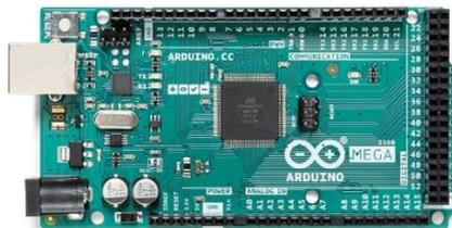
Gambar 2.4 Arduino Mega 2560[7]
