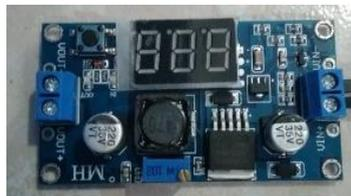
Gambar 2. 6 Modul Step Down LM2596
