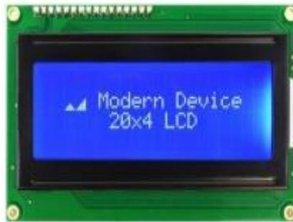
**Gambar 2.4 LCD 20x4**
