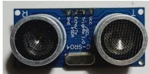
Gambar 2. 3 Sensor Ultrasonik (HC-SR04)
