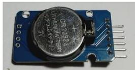
Gambar 2. 4 RTC (*Real Time Clock*)
