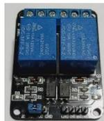
Gambar 2. 6 Relay 2 *channel*
