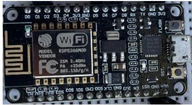
Gambar 2. 8 NodeMCU ESP8266
