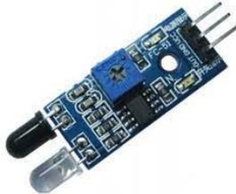
**Gambar 2.9 Sensor *Infrared***
