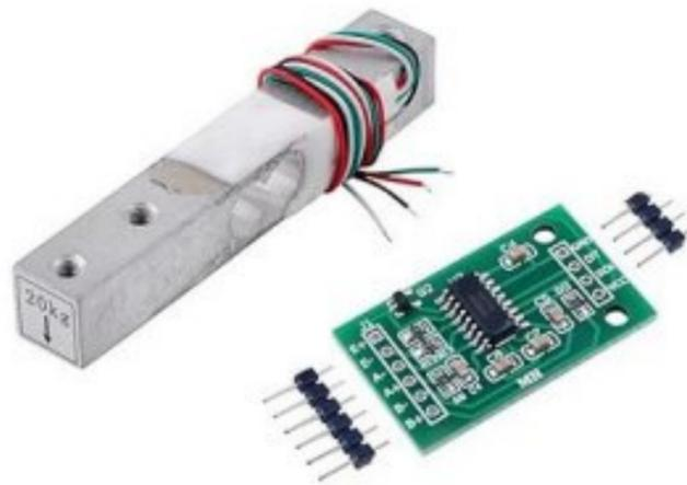
Gambar 2.8 Sensor *Loadcell*
