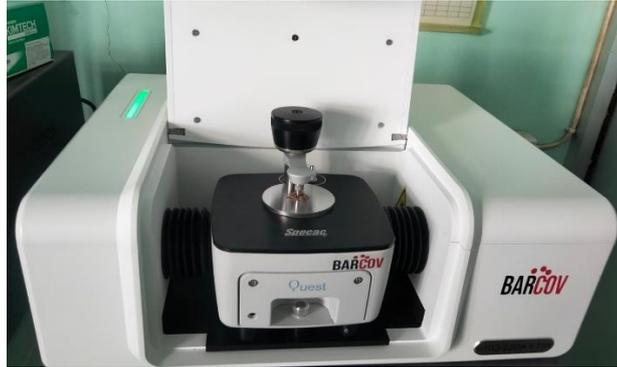
**Gambar 2.5** Instrumen *Fourier Tranform Infra Red (FTIR)* Merk *Barcov* FTIR 530A
