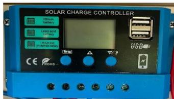
**Gambar 2.3** *Solar Charge Controller*
