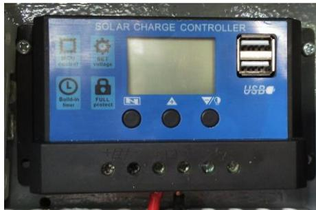
**Gambar 2. 12** *Solar Charge Controller*
