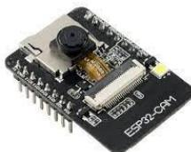
Gambar 2. 3 ESP32 CAM
