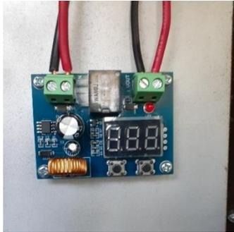
**Gambar 2. 13** Low Voltage Disconnect
