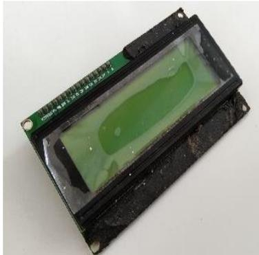
**Gambar 2. 12** *Liquid Crystal Display (LCD)*
