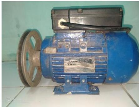
Gambar 2. 1 Motor Asinkron 1 Fasa
