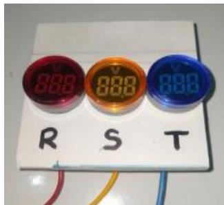
Gambar 2. 8 Voltmeter Digital
