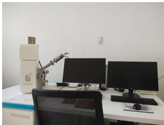
Gambar 2. 5 Instrumen Scanning Electron Microscopy (SEM) (Sumber: Peneliti)
