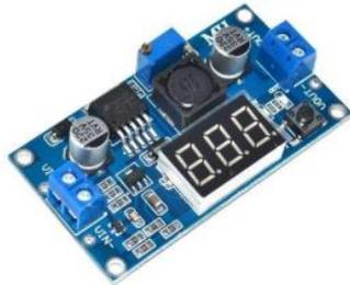
Gambar 2.6 *Step Down DC Buck Converter* LM2596
