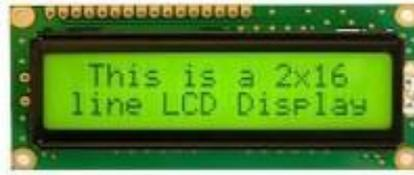
Gambar 2.2 *Liquid Crystal Display 16x2*
