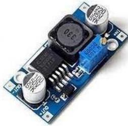
**Gambar 2. 3** modul step down <sup>[25]</sup>
