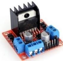
Gambar 2. 5 *Driver Motor L298N*<sup>[25]</sup>
