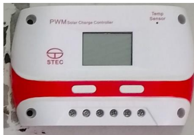
Gambar 2. 2 Solar Charge Controller (SCC)
