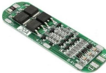
Gambar 2. 8 Battery Management System [12]
