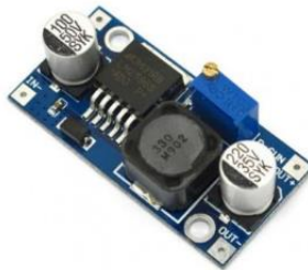
Gambar 2. 7 Modul Step Down [19]
