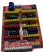
Gambar 2. 2 CNC Shield V3
