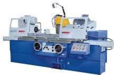
**Gambar 2.3** Mesin Gerinda Silindris (*Cylindrical Grinding Machine*)
