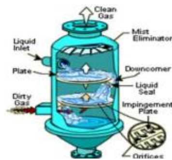
Gambar 2.4 impingement plate scrubbers
