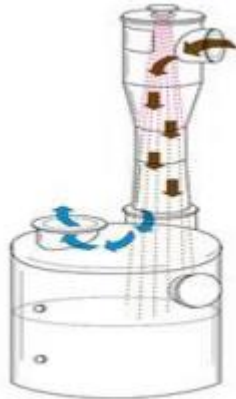
Gambar 2.6 eductor venturi scrubber
