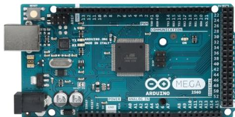
**Gambar 2. 3 Arduino Mega 2560<sup>[16]</sup>**
