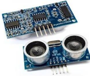
**Gambar 2. 11 Sensor Ultrasonik<sup>[29]</sup>**
