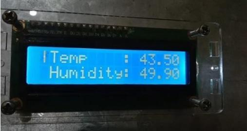
A photograph of a blue LCD screen mounted on a metal frame. The screen displays the text "Temp : 43.50" and "Humidity: 49.90" in white. The screen is backlit, and the entire assembly is held in place by four screws.    |
