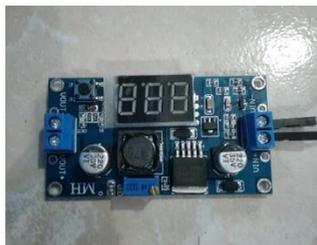
Gambar 2.5 Modul *Step Down* LM2596
