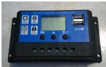
Gambar 2.2 *Solar Charge Controller (SCC)*
