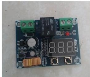
Gambar 2.14 *Low Voltage Disconnect (LVD)*
