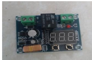
Gambar 2. 4 Low Voltage Disconnect (LVD) (Sumber : Dok. Pribadi, 2023)
