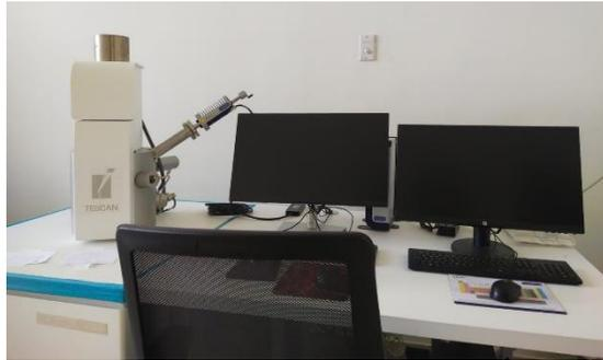
**Gambar 2.5** Instrumentasi *Scanning Electron Microscope* (SEM)
