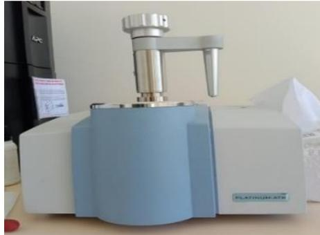
**Gambar 2.4** Instrumentasi *Fourier Transform Infra-Red* (FTIR)
