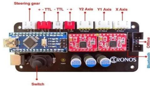
Gambar 2. 7Kontroller Laser CNC 2 Axis
