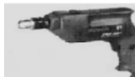
Gambar 2.14 Mesin gurdi portable (Widarto, 2018)
