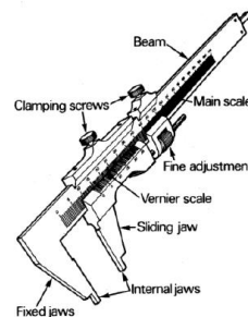
Gambar 2.9 Bagian-bagian jangka sorong (Wirawan, 2008)
