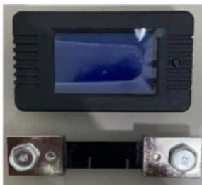
**Gambar 2. 5** Modul Sensor Pzem-015
