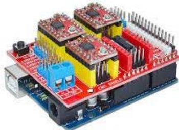
Gambar 2. 2 CNC *Shield* V3 <sup>[9]</sup>
