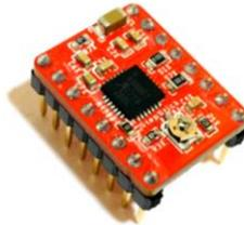
Gambar 2. 3 *Driver Motor A4988* <sup>[10]</sup>
