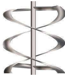
Gambar 2.17 Pengaduk tipe helical ribbon
