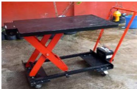
**Gambar 4.1** Desain *electric scissor lift table*
