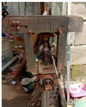
**Gambar 2.13** *Hydraulic pipe bending*
