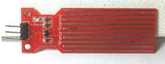
**Gambar 2. 13 Sensor *Water Level***
