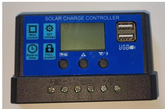
**Gambar 2. 2 Solar Charge Controller**
