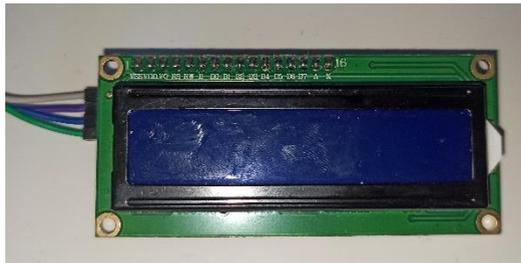
**Gambar 2. 8 LCD 16 x 2**
