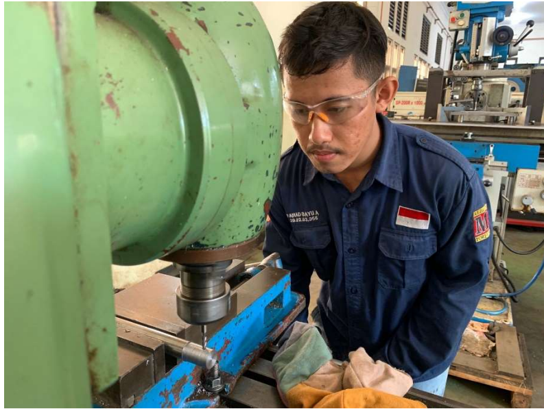
Gambar 6D Proses Frais
