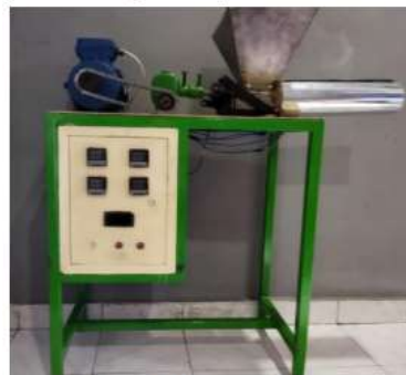
Gambar 2.3 Alat Screw Extruder (Florenza, dkk. 2021)
