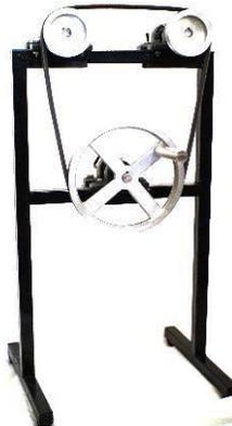
**Gambar 2. 1** Alat pilin serat daun nanas (Millati & Estiyono, 2018)
