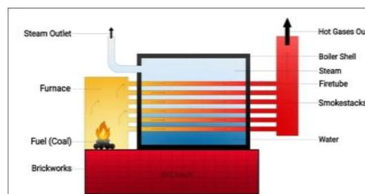
Gambar 2. 1 *Fire tube boiler* ( iqmech, 2021)
