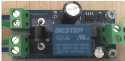
**Gambar 2. 9. Emergency Automatic Switch**
