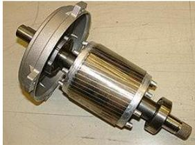
Gambar 2. 5. Rotor Motor
