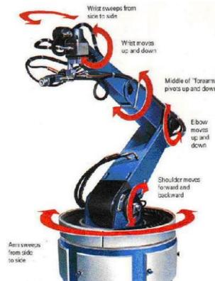
**Gambar 2.4** Gerakan Lengan Robot (Syam, R, 2015)
