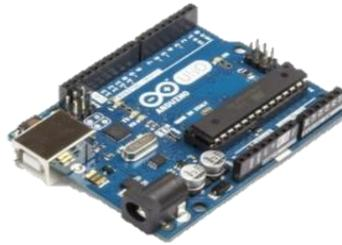
**Gambar 2.5** Papan Arduino Uno (Kadir, A. 2016)
