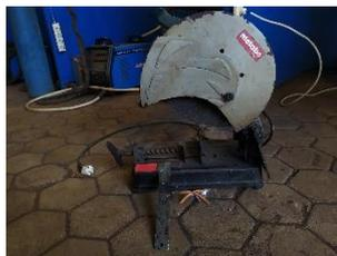
**Gambar 2. 9** Alat potong mesin *metal cutting saw*
